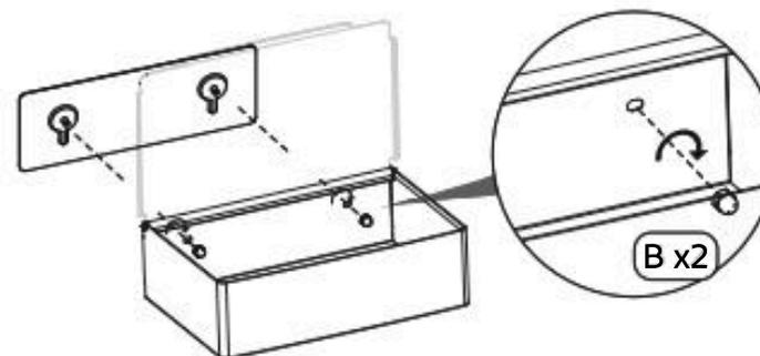
(1b) EN/ Drilled Anchors
